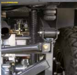
Robust, reliable semi-independent rear suspension
