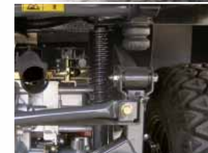
Robust, reliable semi-independent rear suspension
